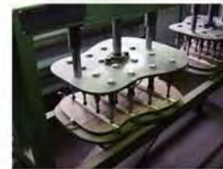
Hydraulic presses hold back bracing and body rims in place.
