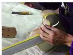
Skilled taping over the binding before painting provides for a clean finish.
