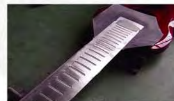
To avoid fretboard damage, this innovative jig provides protection during fret dressing.
