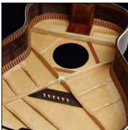
1930s wide-X bracing and deep scarfing on solid-top tone woods are the beginning of these exquisite guitars.
