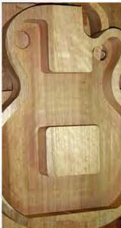
CNC machines make for precision routing of this Kat body.
