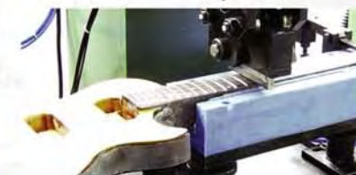
A precision press applies perfect pressure for consistent fret seating.
