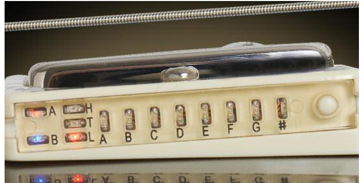
Pickup ring-mounted Chromatic tuner
